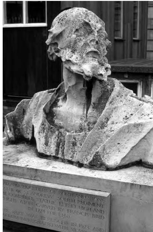
Plate 5.2 A bust of Saint Andrew, removed from St Paul's Cathedral because of accelerated decay.
